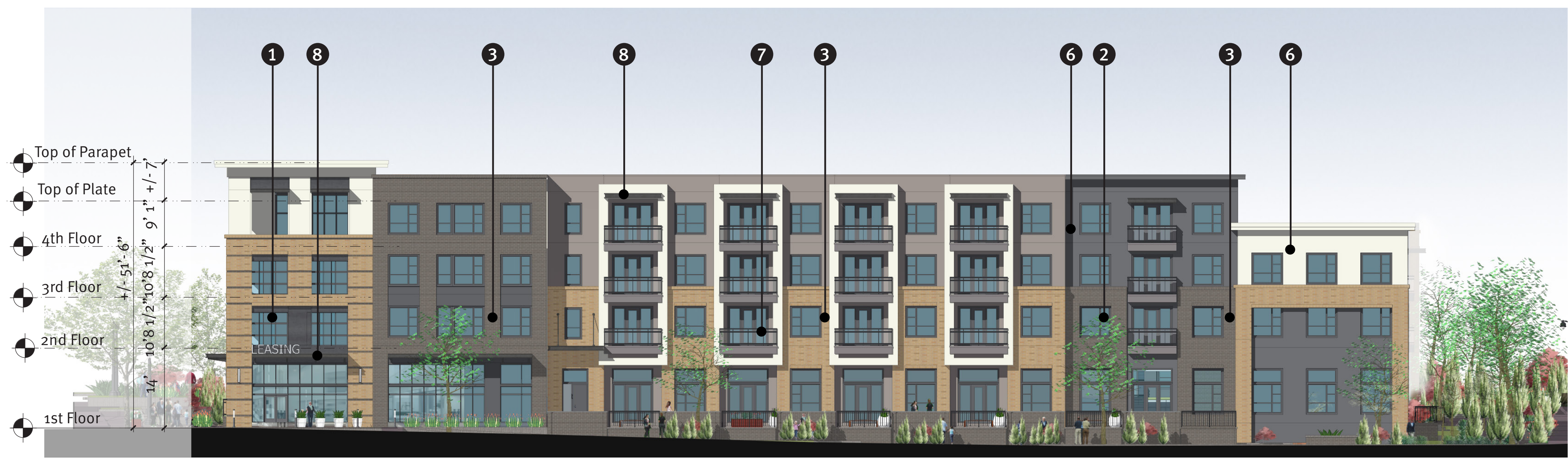
03 East Elevation Exterior Facade Materials: Masonry 100% Percentage of Openings: F1: 35% F2: 37% F3: 37% F4: 28%
